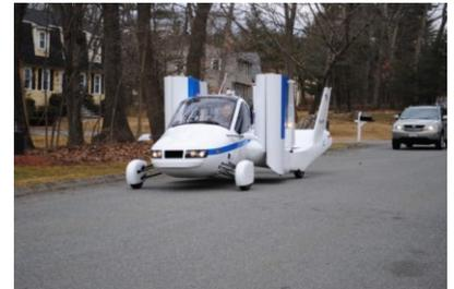
The model pictured above is called The Transition and is billed by the company as "the world's first practical flying car." The company says it runs premium unleaded petrol, fits into a standard single-car garage and converts between flight and drive modes in under a minute. You'll need a Sport Pilot Certificate to lift off the ground, but you can drive it around town with a regular driver's license.
