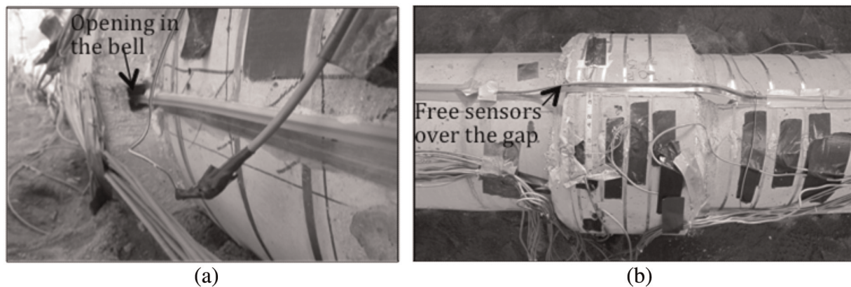
Figure 11. (a) First solution: opening in the bell, Profile sensor (up), and Tape sensor (down) and (b) second solution: free sensors over the gap, Tape sensor (closer), and Cord sensor (farther).
