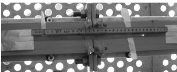
Fig. 10 Crack test 3: delamination from the gap to both sides marked with portion of paper and fibre breakage seen as a glowing spot to the right of the gap
