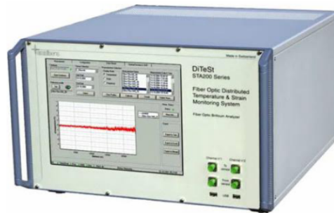
Figure 12 DiTeSt reading unit based on Brillouin backscattering (see online version for colours)
