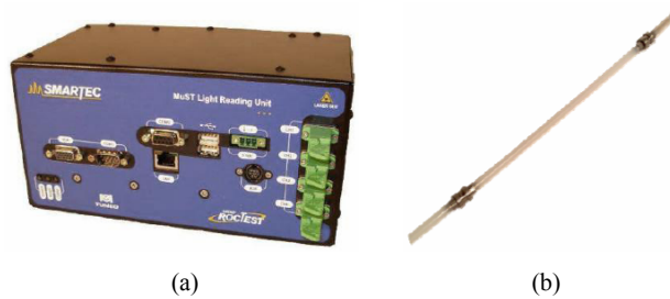
Figure 6 (a) MuST reading unit and (b) MuST deformation sensor (see online version for colours)
