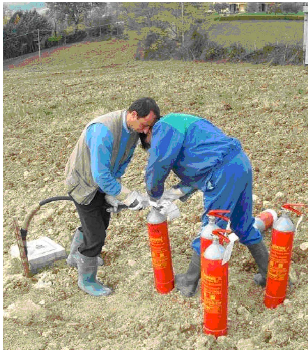
Fig. 11 Leakage simulation test
