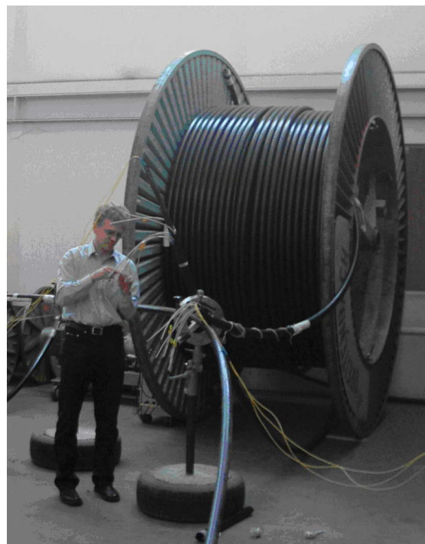
Fig. 18 Liner heating test by electrical current injection
