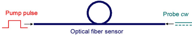
Fig. 1. Schematic of the interaction between probe and pump signals in an SBS-based fiber-optic sensor.
