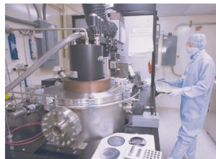
Cutting edge: the plasma etching tool at Cornell is part of the impressive nanotech facility.
