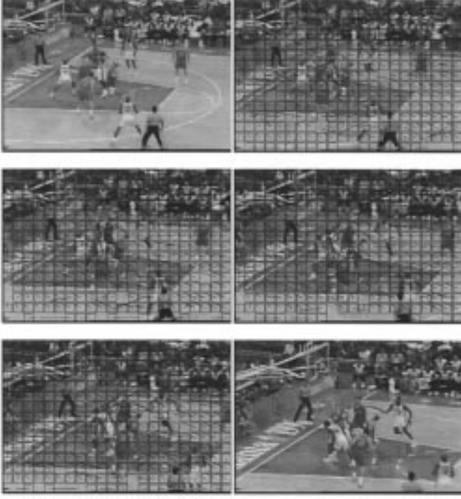
Fig. 4. The initial I -frame and the subsequent P -frames (frames 34, 37, 40, and 43) from the third GOP with GOP sequence IBBPBBPBBPBBPBB from an MPEG video with pan from left to the right, upward tilt, and zoom. For each P -frame, the intercoded motion blocks and the corresponding motion vectors are shown. The last image at the bottom right is the first I -frame of the next GOP.
