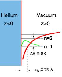
Measurement: Stark-shift transition frequency by field  $E_{\perp}$  to tune microwave radiation to 1- 2 resonance
