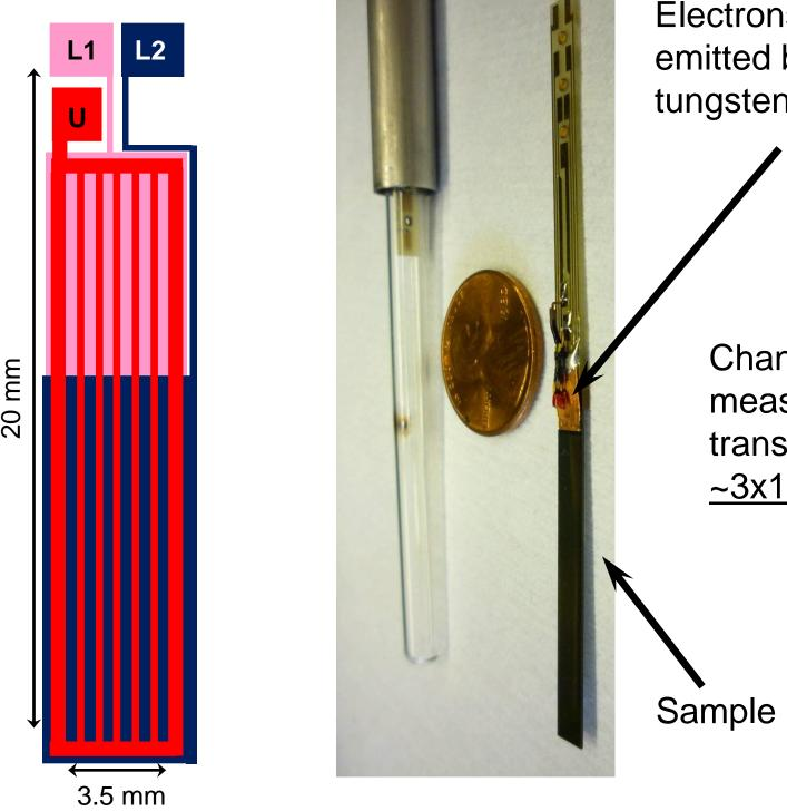
Electrons thermally emitted by tiny tungsten filament Channel population measured by transport to be ~3x10<sup>8</sup> total spins
