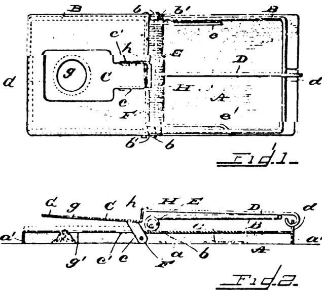
Above--Two figures were submitted for U.S. Patent No. 661,068, the mousetrap, which was issued in 1900. The invention is "a trap of simple construction which can be manufactured inexpensively" in which "the bait cannot be removed without releasing the engaging jaw."
