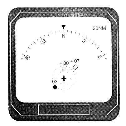
Traffic may be displayed on a CRT system, such as a dedicated display, a weather radar, or an electronic flight instrument system.
