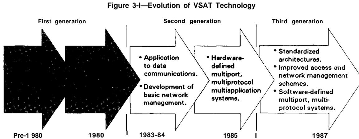
The evolution of very small aperture terminal (VSAT) technology: three generations.
