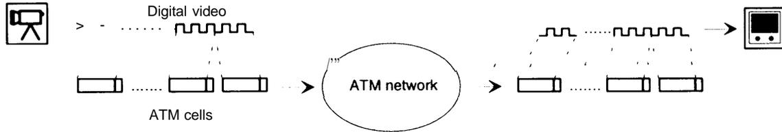
The digital video bits are put in cells and sent through the network. At the destination, the bits are removed from the cells.
