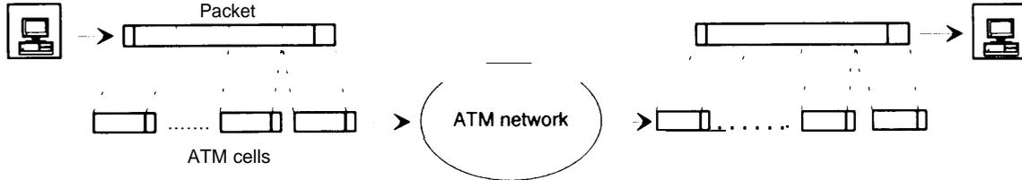
Packets are broken into several ATM cells. After traveling through the network, the cells are reassembled into packets.
