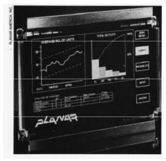
Medical, industrial, and transportation systems require the display of bright, sharp images in a rugged package, such as this electroluminescent display
