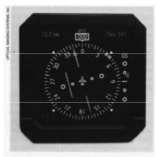
Flat panel displays present video and fright instrumentation date in cockpit avionics using a fraction of the space and weight of cathode ray tubes and electromechanical displays.
