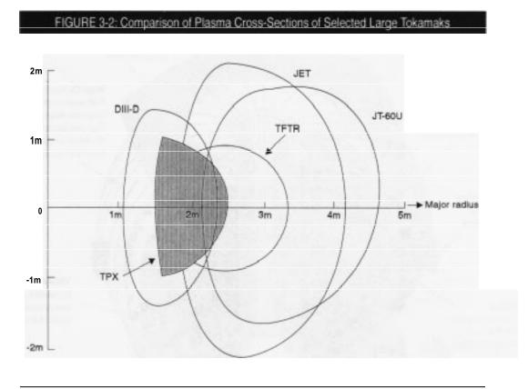
DIII-D = General Atomics, USA; JET = Joint European Torus, European Community, Culham Laboratory, U. K.; JT-60U = JT-60 Upgrade, Japanese Atomic Energy Research Institute, Japan; TFTR = Tokamak Fusion Test Reactor, Princeton Plasma Physics Laboratory, USA; TPX = Tokamak Plasma Experiment, Princeton Plasma Physics Laboratory, USA SOURCE: Office of Technology Assessment, 1995, based on a figure provided by David Overskei, General Atomics.
