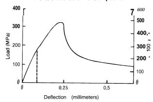
Dotted line indicates deflection at which a single crack has passed completely through the matrix, but remains bridged by intact fibers,
