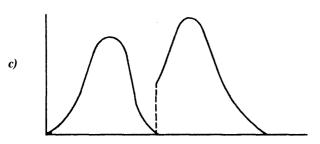
The probability of failure of a ceramic component is the overlap between the applied stress distribution and the material strength distribution, as shown in (a). This probability can be reduced by reducing the flaw size (b), or truncation of the strength distribution through proof testing (c).
