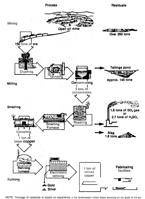
Figure 1.1 — Principal Stages of the Copper Production Process
