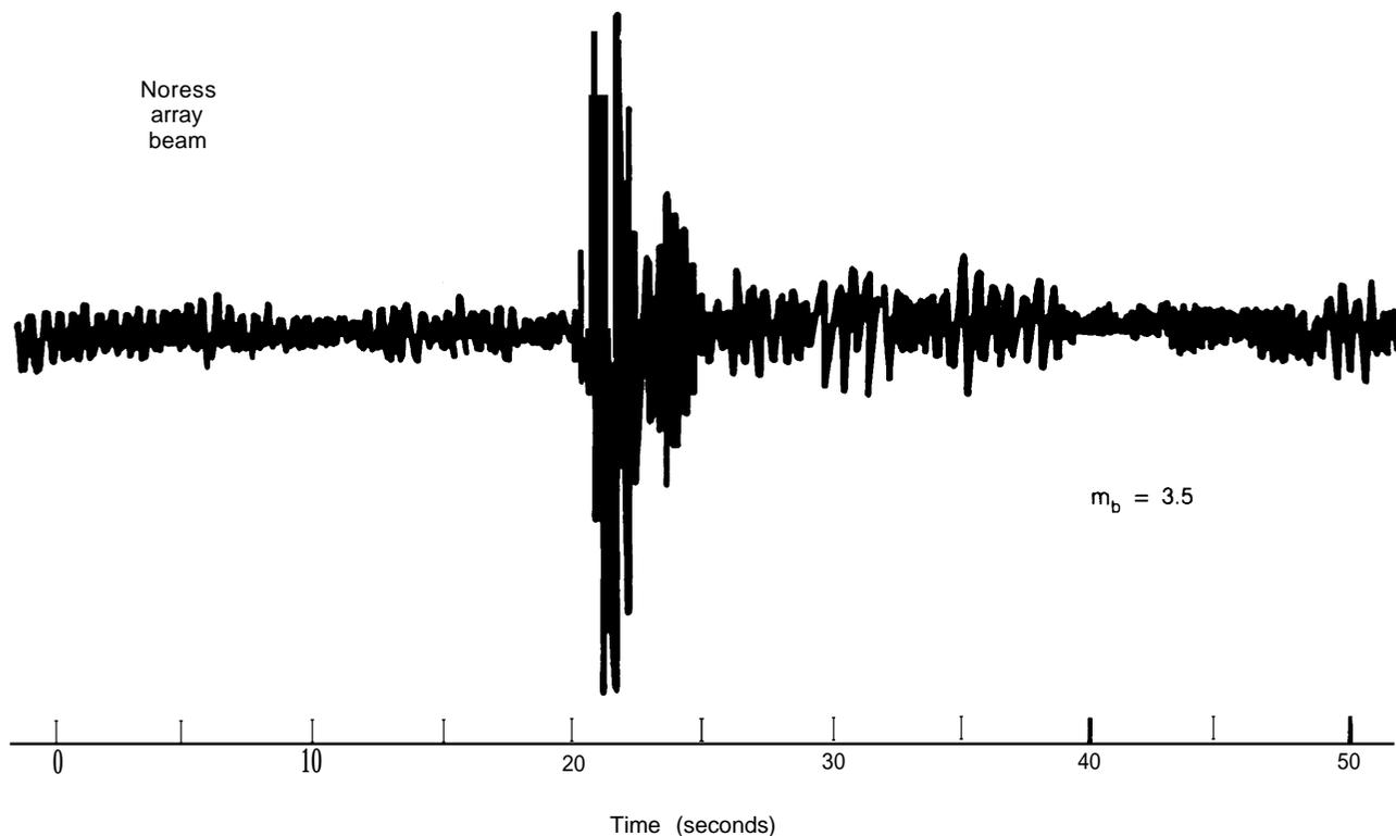
Seismic signal from a 0.25 kt explosion at the Soviet test site near Semipalatinsk. Recorded 3,800 km away at the NORESS seismic array in Norway on July 11, 1985. The signal to noise ratio is about 30 indicating that much smaller explosions could be detected even at this great distance.
