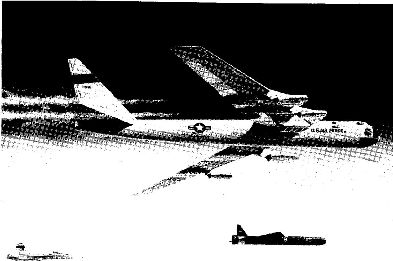
The Pegasus air-launched vehicle is released from a modified B-52 aircraft operated by NASA's Dryden Flight Research Facility (artist's concept).
