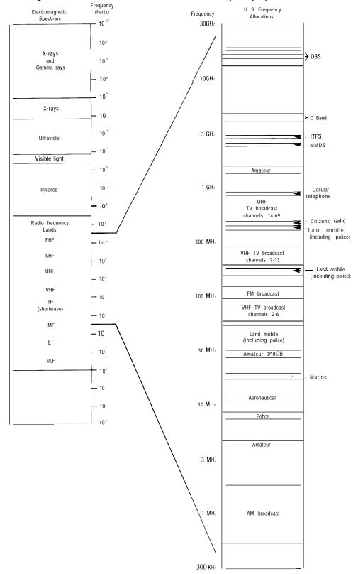
Figure 3-4-Selected Allocations of the Radio Frequency Spectrum
