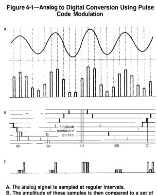
B. The amplitude of these samples is then compared to a set of discrete amplitude steps and converted into numerical values. These values are shown written in binary.
