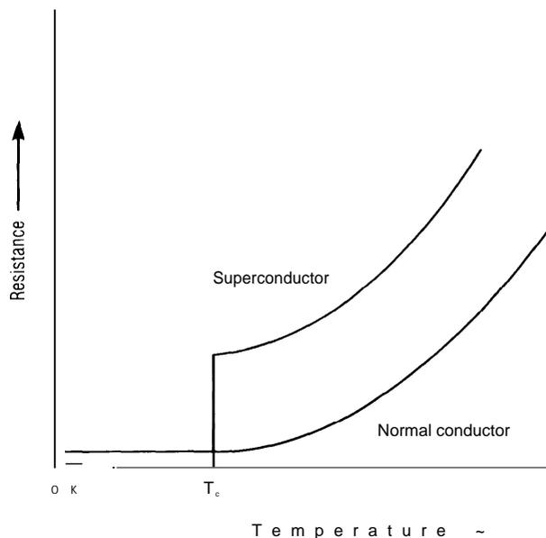
At  $T_c$ , the resistance of a superconductor drops to zero.
