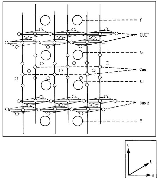
The supercurrent is carried primarily in the  $\text{CuO}_2$  planes.
