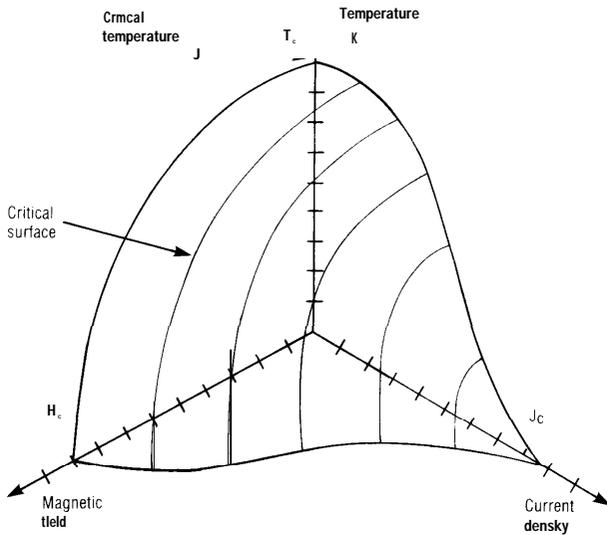
Material must be maintained below the "critical surface" to remain superconducting.
