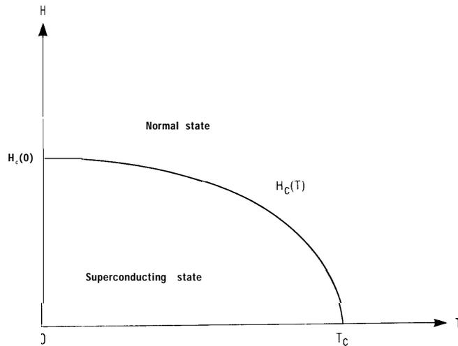
Material must be at field and temperature below the  $H_c(T)$  line to remain superconducting.
