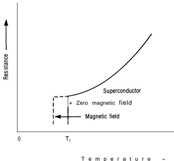
An applied magnetic field causes resistance to appear in HTS materials below  $T_c$ .
