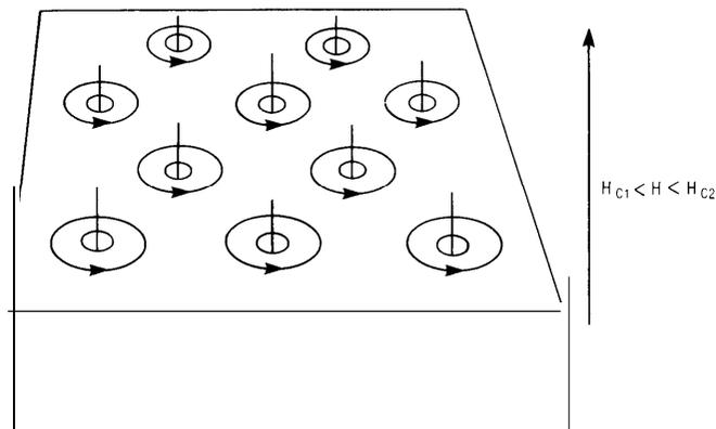
When the applied magnetic field is between  $H_{c1}$  and  $H_{c2}$ , lines of magnetic flux penetrate the superconductor, surrounded by supercurrent "whirlpools." As long as these flux lines remain "pinned" at fixed sites, the superconductivity is not impaired.
