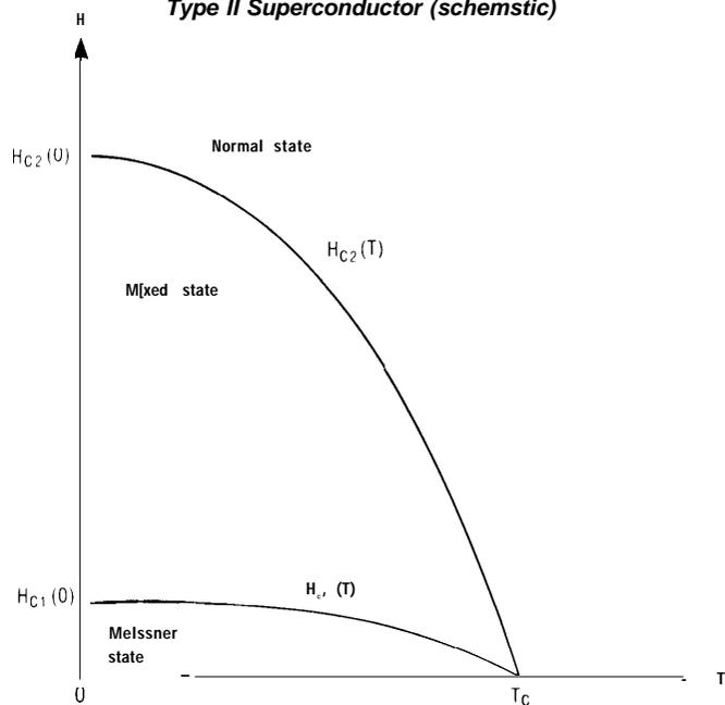
Magnetic flux lines enter the material for fields above  $H_{c1}(T)$ . Material remains superconducting below upper critical field  $H_{c2}(T)$ .
