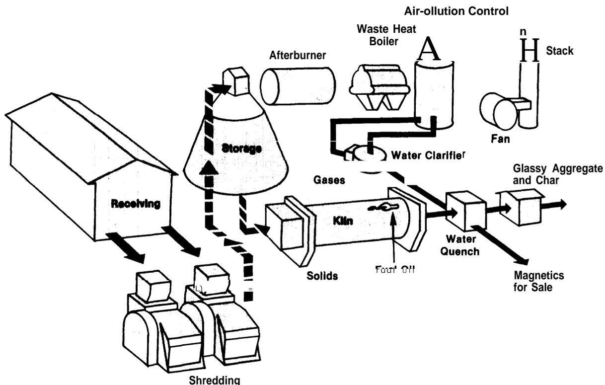
Figure C\*5.—Torrax Slagging Pyrolysis System
