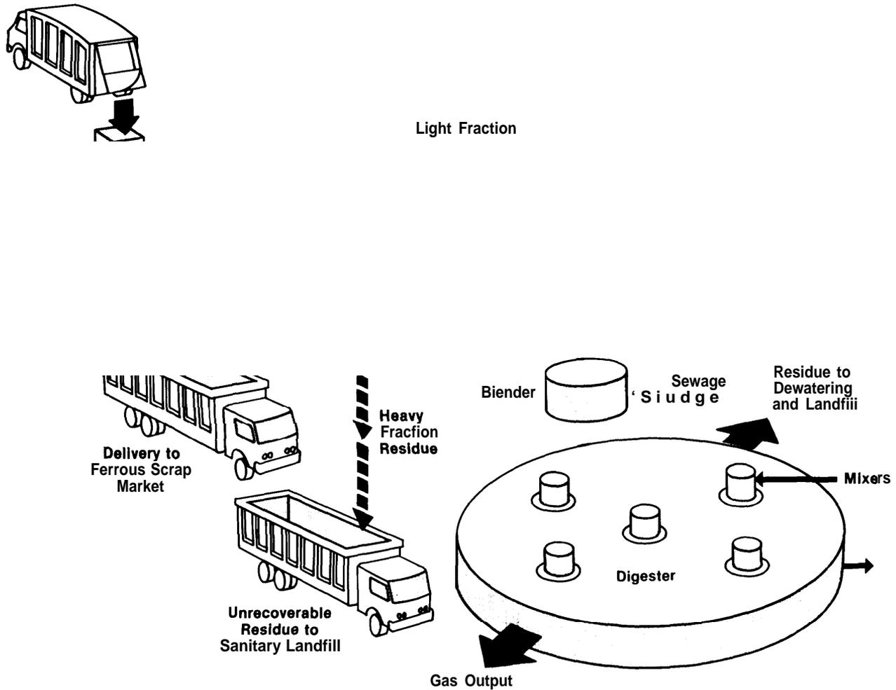
ing tanks, with the remainder discharged to a city sanitary sewer system. The remaining solids, about 17 percent of the refuse feed, must be either landfilled or burned in specially designed boilers. Schulz (6) estimates that approximately 3,700 cubic feet of methane will be produced per ton of MSW.
