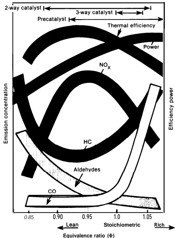
The equivalence ratio is the ratio of the A/F ratio which is exactly sufficient to completely burn all of the fuel to the actual A/F ratio used in the car. Leaner mixtures have an excess of air, while richer ones have an excess of fuel.
