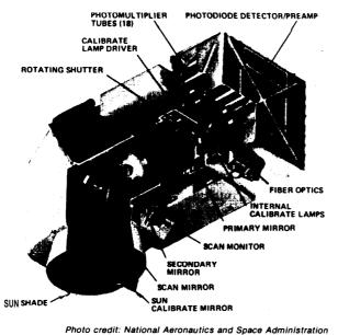
Cutaway view of the multispectral scanning system
