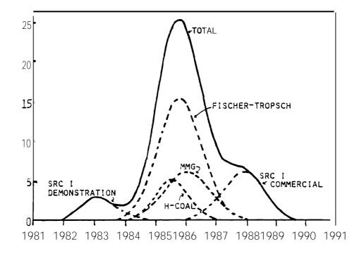
Figure 5-2: Synfuel plant construction labor requirement near Owensboro, Kentucky.
