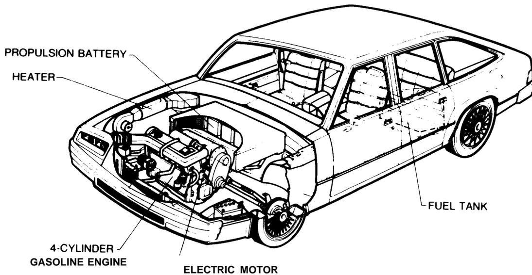
Figure 4.5 Schematic of DOE's Hybrid Test Vehicle HTV-1
