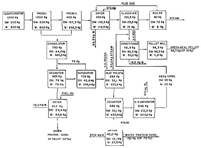
Figure 24.—Material Flow in Vepex Process
