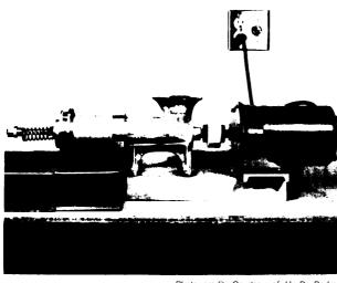
Figure 5.— Rebuilt Meat Grinder as Miniature Screw Press
