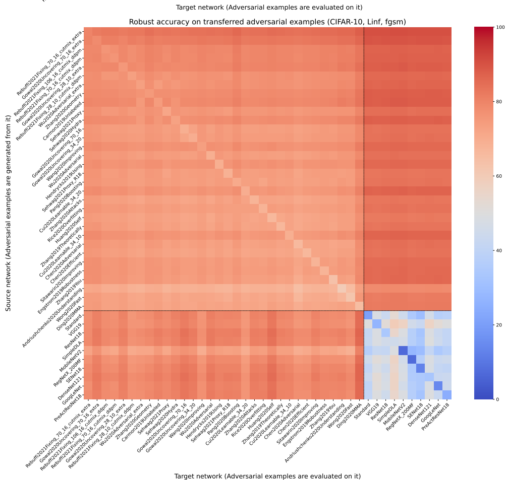
Figure 18: Measuring transferability of adversarial examples ( \ell_\infty , \epsilon = 8/255 ). We use a ten step PGD attack in top figure and FGSM attack in bottom figure. Lower robust accuracy implies better transferability.
