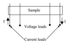
voltage will be proportional to the resistance of the sample and will be independent of the wire and/or contact resistance. If the sample is superconducting, the voltage between the voltage leads should be exactly equal to zero.
