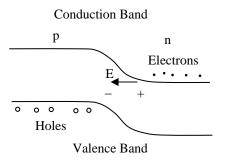
release energy equal to the band gap. This energy can be emitted as a photon. Conversely, an electron-hole pair can be created by a photon, as used in photodiodes to detect light.
