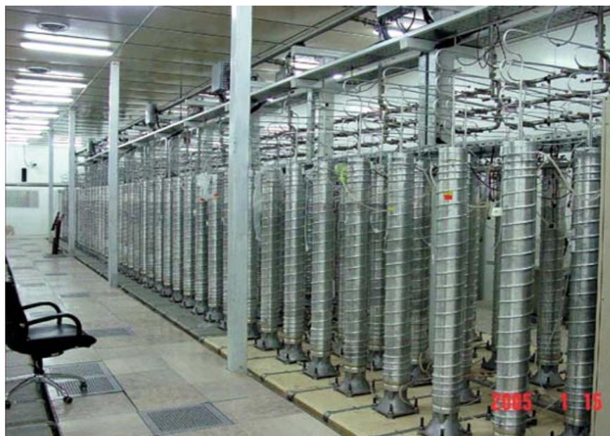
**Figure 3.** The first publicly released picture of the 164-machine cascade installed at Iran's aboveground Pilot Fuel Enrichment Plant. The photo was used in a presentation by Mohammad Saeidi of the Atomic Energy Organization of Iran in September 2005.
