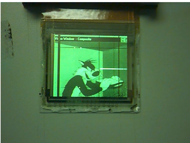
Fig. 9. QVGA Display showing video operation.
