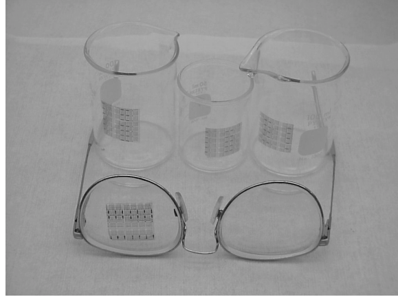
Figure 4. TFT structures on thin plastic substrates and attached to curved surfaces.
