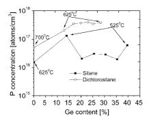
**Figure 2.** N-type background doping for both silane and dichlorosilane silicon sources as a function of germanium content; the growth temperatures ranged from  $525\,^{\circ}\text{C}$  to  $700\,^{\circ}\text{C}$ , with a growth pressure of 6 Torr and a hydrogen carrier of 3 slpm. The silane flow was  $10\,\text{sccm}$  and the dichlorosilane flow was  $6.5\,\text{sccm}$ .
