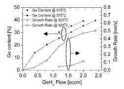
**Figure 3.** Growth rate and Ge concentration versus germane flow rate using silane as a precursor at 525 °C and 575 °C. The pressure is 6 Torr with a 3 slpm hydrogen carrier, and the silane flow is 10 sccm.
