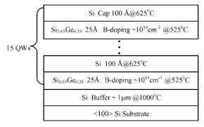
Figure 4. Cross section of the targeted sample structure.
