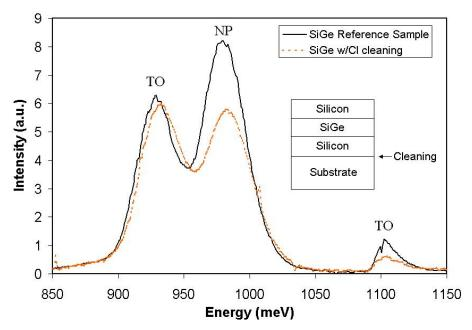
Figure 6 Photoluminesence intensity vs. photon energy at  $77^{\circ}$ K. Indicated on the plot are the TO (transverse optical phonon replica) for Si and SiGe and the NP (no phonon) peaks for SiGe. Photoluminesence for a reference SiGe quantum well with a 1000°C bake in hydrogen instead of a Cl<sub>2</sub> etching step is compared with the structure with Cl<sub>2</sub> etching of the substrate.
