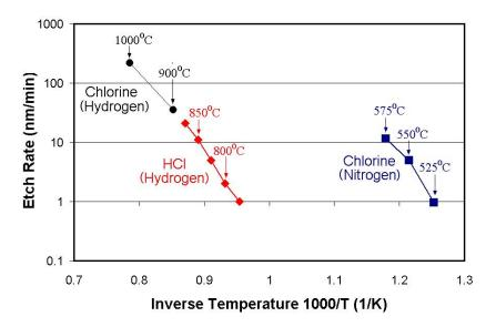
Figure 1 Etch rate of <100> silicon surface versus inverse temperature. Etch conditions using chlorine were 3 slpm of nitrogen or hydrogen flow and 15 sccm of chlorine flow at a pressure of 6 torr, for a chlorine partial pressure of 30 mtorr. HCl etch rates in hydrogen are from Ref. 3; the partial pressure of HCl is 200 mtorr with a hydrogen partial pressure of 20 torr.
