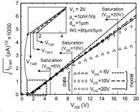
**Fig.7.** Variation of  $V_{Ta}$  for different drain biases. Reducing  $V_{DS}$  shrinks the saturation regime over which the LSF is calculated. The extracted  $V_{Ta}$  (and  $\mu_{na}$ ) increases with reducing the drain bias as predicted by the model.
