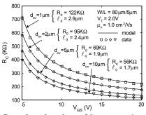
**Fig.4.** Gate voltage dependence of the contact resistance  $R_C$  for various gate to drain/source overlap  $d_{ov}$ . The  $R_C$  values are extracted from the I-V curve of the test TFTs following the approach introduced in [2].
