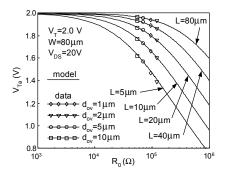
**Fig.6.** Variation of  $V_{Ta}$  versus  $R_0$  for several values of channel length, *L*. The extracted  $V_{Ta}$  is lower at shorter *L* and higher  $R_0$ , as predicted by the model.
