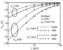
**Fig.8.** Variation of  $V_{Ta}$  versus L for two  $d_{ov}$  and  $V_{DS}$  values and comparison with the model. The extracted  $V_{Ta}$  is lower at shorter L, higher  $R_0$  and higher  $V_{DS}$ , as predicted by the model.
