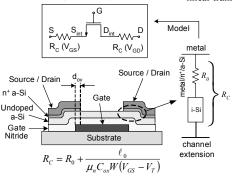
**Fig.3.** Cross-section of an inverted-staggered a-Si TFT. The contact resistance  $R_C$  is composed of a metal/n<sup>+</sup>Si/a-Si metallurgical junction and an a-Si region beneath that junction. The latter component makes  $R_C$  gate-voltage dependent [2].
