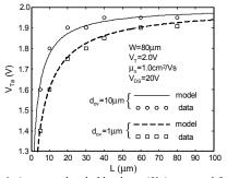
**Fig.1.** Apparent threshold voltage ( $V_{Ta}$ ) extracted from test TFT's using the conventional method, for several channel lengths (L) and two gate to drain/source overlap lengths,  $d_{ov}$  (see Fig. 3). The shorter  $d_{ov}$  corresponds to the higher contact resistance. It is observed that  $V_{Ta}$  is lower at shorter L and also lower for higher contact resistance (shorter  $d_{ov}$ ).
