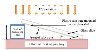
Figure 4 Schematic indicating the loading sequence in SA-2 and SA-3
