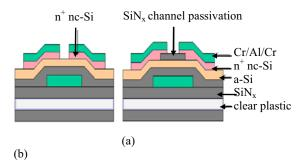
**Figure 2** a-Si:H TFT structures: (a) back-channel cut, bottom-gate staggered source-drain, (b) back-channel
