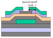
Figure 3 Schematic cross section indicating the critical overlaps (1) and (2) for bottom-gate back-channel passivated a-Si:H TFTs
