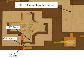
Figure 7 Optical micrograph of a back-channel passivated TFT fabricated using SA-3 at 300°C on clear plastic. The TFT W/L is 360 μm / 3 μm.
