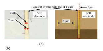
Figure 6 Optical micrograph of the channel region of backchannel passivated TFTs fabricated using SA-3, on clear plastic, with channel lengths of (a)  $L = 5\mu m$  and (b)  $L = 3\mu m$ . The maximum process temperature was 300°C
