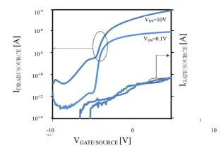
**Figure 8** Transfer characteristics of an a-Si:H TFT fabricated at 300°C using a back-channel passivated geometry and SA-3 self-alignment
