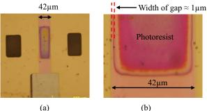
Figure 5 A TFT after the source-drain self-alignment step (a) whole TFT (b) close-up of channel region, showing the 1µm gap between the edge of the gate and the photoresist created using SA-2. The W/L of this TFT is designed to be 80µm/40µm
