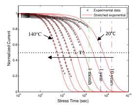
Fig. 2 Current degradation measured from 20°C to 140°C in steps of 20°C, and unified stretched exponential fit to experimental data.
