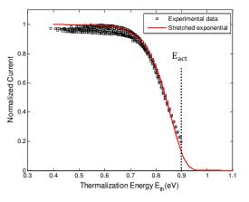
Fig. 3 Normalized drain current unified with thermalization energy  $E_{th} = kTln(vt)$ , where  $v = 5 \times 10^{6}$  Hz,  $E_{act} = 0.9$ eV and  $T_{0} = 643$ K.
