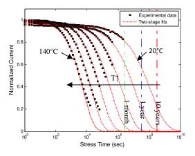
Fig. 5 Two-stage (Stage I + Stage II) fits to drain current degradation from 20°C to 140°C.
