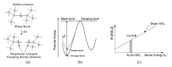
Fig. 1 Defect creation in a-Si TFTs. (a) Defect creation mechanism; (b) configuration coordinate diagram of defect creation and (c) density of weak bonds with barrier energy  $E_b$  modeled with  $n(E) \propto e^{E_b/kT_0}$ . From time t to t + dt, we approximate that weak bonds with barrier energies from  $E_{th}$  to  $E_{th}$  +  $dE_{th}$  all break into dangling bonds (shaded area).
