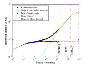
Fig. 4 Two-stage fit to threshold voltage shift vs. time at 20°C. The blue squares for Stage I "data" result from subtracting the Stage II model (determined by high temperature experiments) from the experimental data
