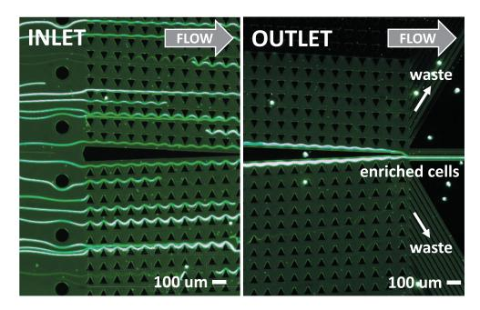
FIG. 3. **CTC** enrichment in **DLD** array. Trajectories of GFP-expressing MDAMB231 breast cells in an array with 42  $\mu m$  gaps, 1/20 array tilt, and 7  $\mu m$  critical particle size at device inlet and outlet at flow rate of 500  $\mu L/min$ . Cells are evenly dispersed at inlet but are concentrated against central wall at outlet and directed to narrow collection outlet.
