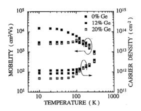
FIG. 1. Temperature-dependent Hall measurements for three samples with 0%, 12%, and 20% germanium in the 75 Å quantum well. All samples had a nominal 100 Å spacer and a  $10^{19}$  cm<sup>-3</sup>  $n^+$  cap layer.
