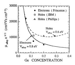
FIG. 4. Calculated alloy scattering limited mobility (in cm<sup>2</sup>/V s) of electrons ( $V_{alloy}=0.8 \text{ eV}$ ) and holes ( $V_{alloy}=0.6 \text{ eV}$ ), normalized by the carrier concentration (in  $10^{11} \text{ cm}^{-2}$ ) as a function of germanium content. The solid squares are experimental data from Table I while the open symbols represent maximum low temperature hole mobilities reported in Refs. 3 and 4.
