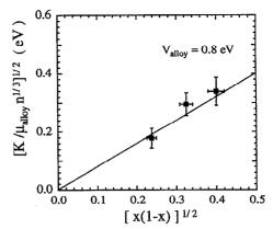
FIG. 2. Alloy scattering model calculations displayed with  $V_{\text{alloy}}$  as an independent parameter. K is a material dependent parameter defined in the text, while  $\mu_{\text{alloy}}$ , n, and x are experimental values from Table I. The data are best fit by  $V_{\text{alloy}} = 0.8 \pm 0.1$  eV given by the slope of the solid line.
