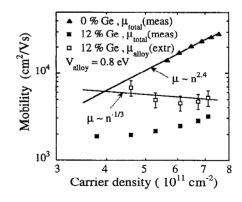
FIG. 3. Mobility as a function of carrier concentration for two similar structures with 0% and 12% Ge quantum wells. Solid triangles and squares are measured data while open squares are extracted alloy mobilities after subtracting impurity scattering. Lines represent best fits to the data given by  $\mu \sim n^{2.4}$  for impurity scattering and  $\mu \sim n^{-1/3}$  for alloy scattering.
