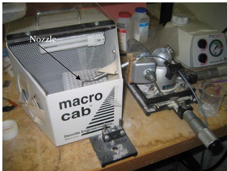
Figure 4-2: The setup used for sandblasting holes through the silicon wafer, to allow fluid and cells to enter and leave the device from the back.
