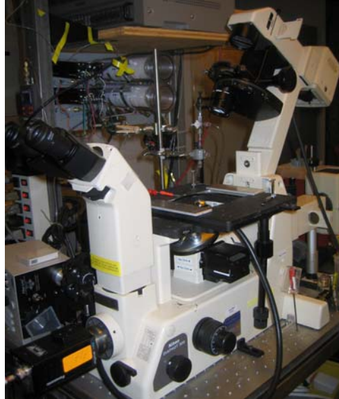
Figure 4-4: The microscope setup used herein. The device in a chuck is placed on the stage of the inverted microscope. Fluidic connections are made from the top. The CCD camera is visible in the lower left corner.
