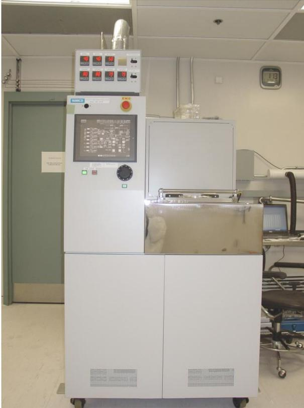
Figure 1. The main unit of the PRISM MNFL Samco RIE200iP etcher.
