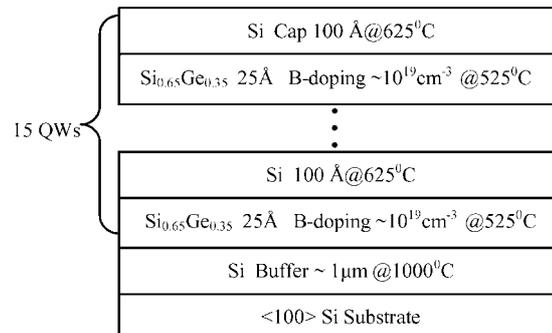
**Figure 4.** Cross section of the targeted sample structure.
