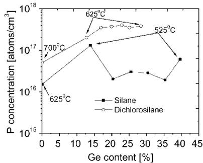
**Figure 2.** N-type background doping for both silane and dichlorosilane silicon sources as a function of germanium content; the growth temperatures ranged from 525 °C to 700 °C, with a growth pressure of 6 Torr and a hydrogen carrier of 3 slpm. The silane flow was 10 sccm and the dichlorosilane flow was 6.5 sccm.
