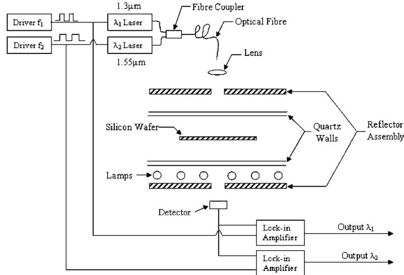
**Figure 1.** Schematic diagram of the rapid thermal processing system adapted for infrared transmission measurements [8].
