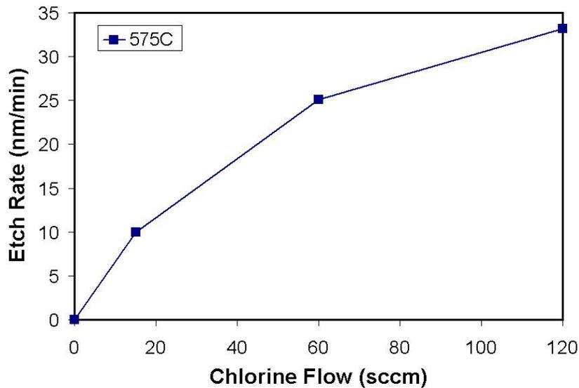
Figure 2 Etch rate of <100> silicon surface versus chlorine flow rate at 575°C. The pressure was 6 torr with 3 slpm of nitrogen flow.
