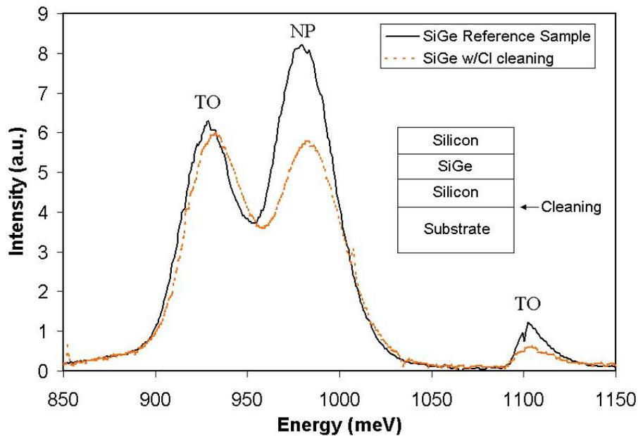
Figure 6 Photoluminescence intensity vs. photon energy at 77°K. Indicated on the plot are the TO (transverse optical phonon replica) for Si and SiGe and the NP (no phonon) peaks for SiGe. Photoluminescence for a reference SiGe quantum well with a 1000°C bake in hydrogen instead of a Cl<sub>2</sub> etching step is compared with the structure with Cl<sub>2</sub> etching of the substrate.
