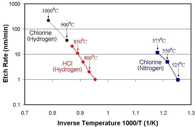
Figure 1 Etch rate of <100> silicon surface versus inverse temperature. Etch conditions using chlorine were 3 slpm of nitrogen or hydrogen flow and 15 sccm of chlorine flow at a pressure of 6 torr, for a chlorine partial pressure of 30 mtorr. HCl etch rates in hydrogen are from Ref. 3; the partial pressure of HCl is 200 mtorr with a hydrogen partial pressure of 20 torr.
