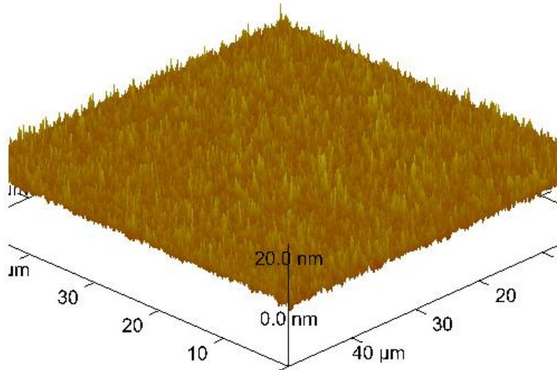
Figure 3 AFM image of silicon surface after etching of 20nm of silicon at 575°C and a pressure of 6 torr with a flow of 15 sccm of chlorine.
