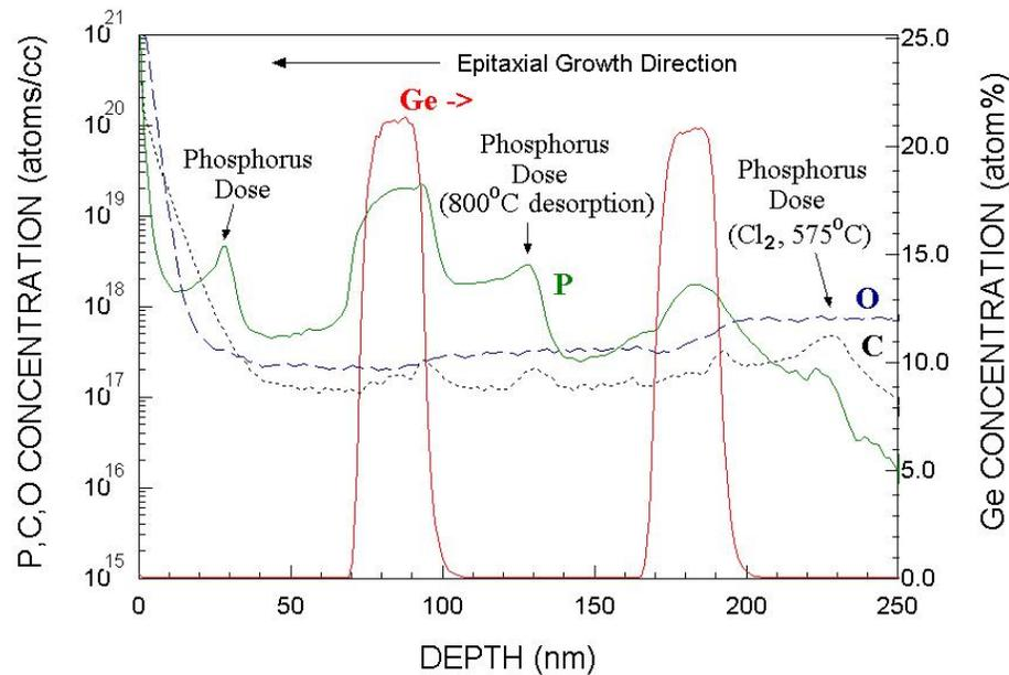
Figure 5 Secondary Ion Mass Spectrometry plotting depth versus impurity concentration for P (solid), C (dotted), and O (dashed). Growth was halted to cover the surface with phosphorus by injecting phosphine into the chamber at 3 different times during the growth. After the first two phosphine doses, different techniques were used to attempt to remove the phosphorus from the surface. SiGe layers were grown in between phosphorus doses to reduce the surface phosphorus concentration.
