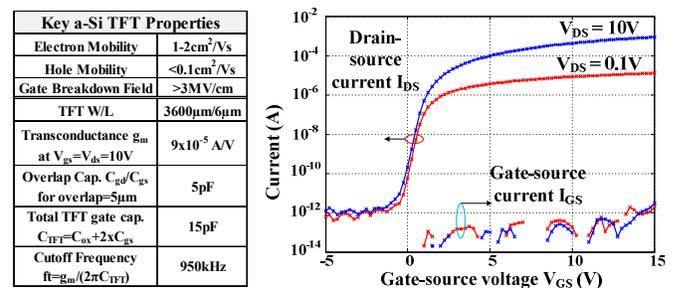
Fig. 2: a-Si TFT device properties lead to typical  $f_i$  of approximately 1MHz due to low  $g_m$  and large parasitic gate capacitances.
