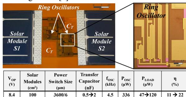
Fig. 11: Prototype of capacitive energy harvesting block with typical performance achieved [1]. Inset shows ring oscillator which generates the control signal for either M1 or M2.
