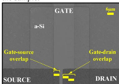
(a) TFT on  $50\mu m$  polyimide, with all layers processed below  $180^\circ C$ .
