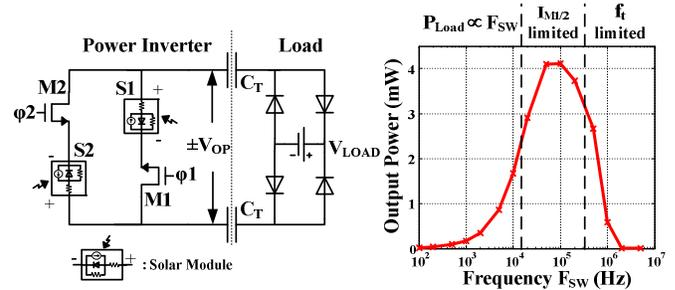
Fig. 5: Class-D power-transfer stage, achieving switching using only NMOS devices [1]. Plot shows output power scaling with frequency.
