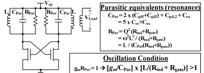
Fig. 6: Resonant Class-A power stage; resonant operation requires meeting a positive-feedback condition.
