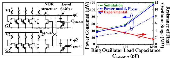
Fig. 10: Improvement of power-efficiency (at constant oscillator frequency) can be achieved through reduction of C<sub>gate-M1/2</sub> which allows for oscillator load resistance scaling. Power results are shown from simulation, a static power model and experimental measurements.
