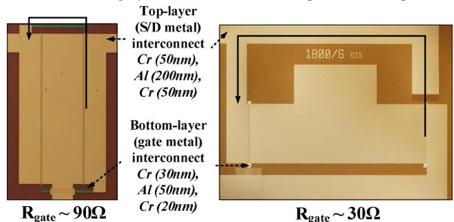
(b) Layout effects on gate resistance  $R_{gate}$ , with cross-coupling achieved using the bottom gate metal layer (left) or the top S/D metal layer (right).
