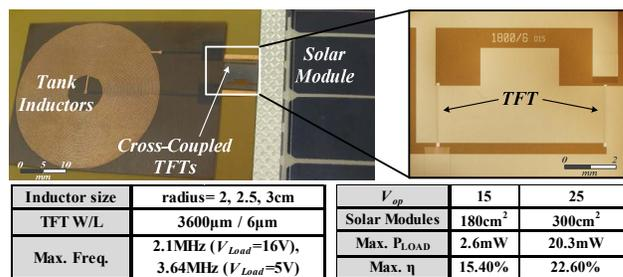
Fig. 12: Prototype of inductive energy harvesting block with typical performance above f, shown [2]. Inset shows tank TFTs.
