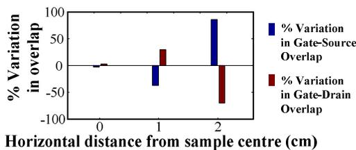
(b) Source and Drain overlap variation across a sample due to substrate deformation.
