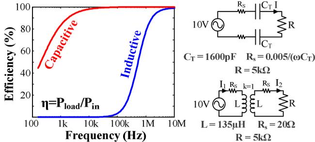
Fig. 4: Efficiency of capacitive vs. inductive power-transfer stages.
