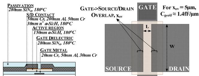
Fig. 1: Thin-Film Transistor (TFT) side and top views.
