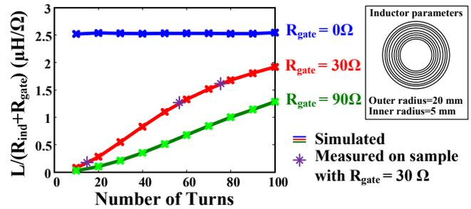
Fig. 8: Patterned inductor  $L/R$  ratio dependence on number of turns with and without effect of  $R_{gate}$ . Simulated results obtained using [6].
