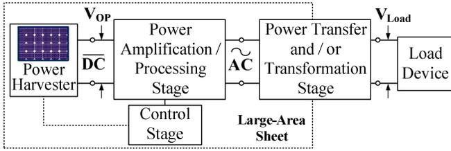
Fig. 3: Power inversion system as a representative application for thin-film power circuits.
