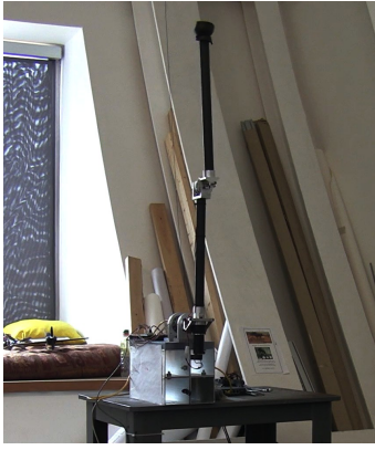
Fig. 4: Picture of the Acrobot balancing in the upright configuration using the controller designed with SDSOS programming. A video of the controller in action is available online at https://www.youtube.com/watch?v=FeCwtvrD76I .
