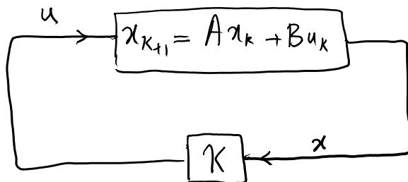
This is a basic problem in control theory. In the controls jargon, we would like to design linear controller  $u = Kx$  which is in feedback with a "plant"  $x_{k+1} = Ax_k + Bu_k$  and makes the closed-loop system stable:
