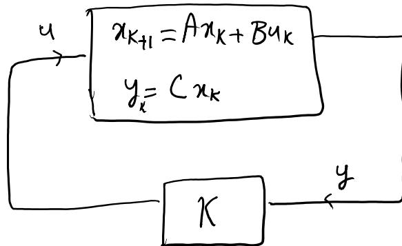
This problem is similar to our previous one, except that instead of feeding back the full state  $x$  to the controller  $K$ , we feed back an output  $y$  which is obtained from a (possibly non-invertible) linear mapping  $C$  from  $x$ . For this reason, the question of existence of a  $K$  that makes the closed-loop system (i.e.,  $A + BKC$ ) stable is known as the "stabilization with output feedback" problem.
