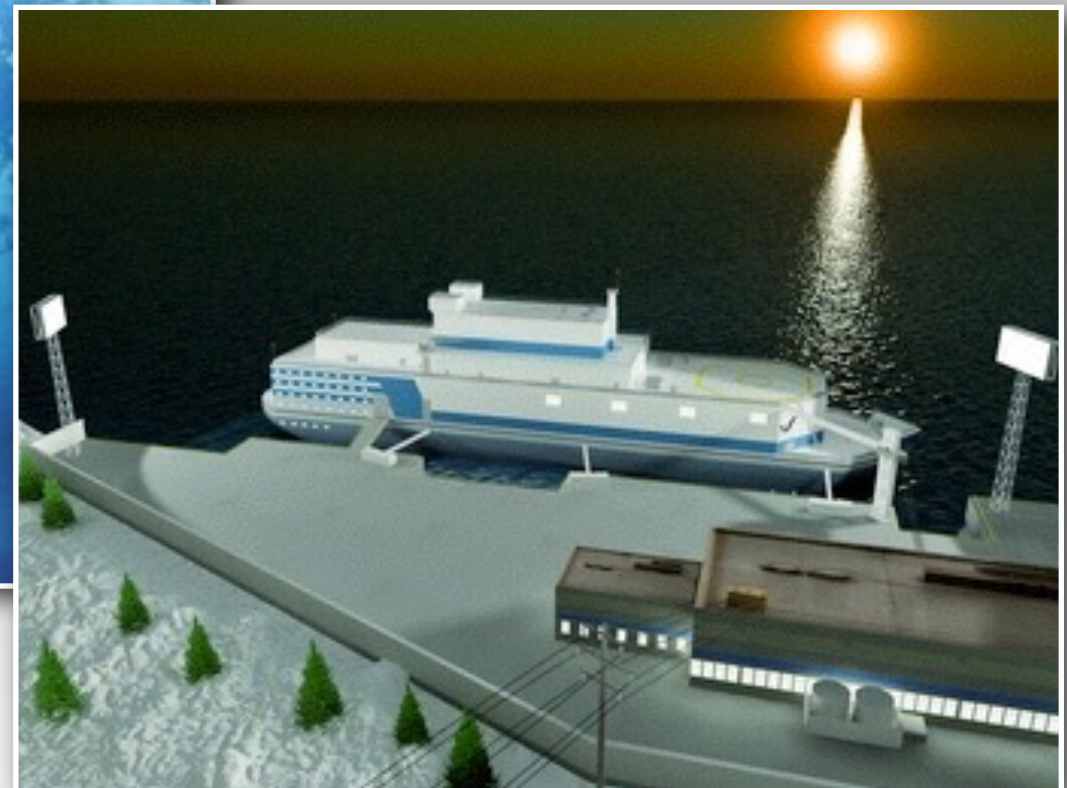
Floating Nuclear Power Plant proposed by Rosatom Akademik Lomonosov (2 x 32 MWe) under construction
