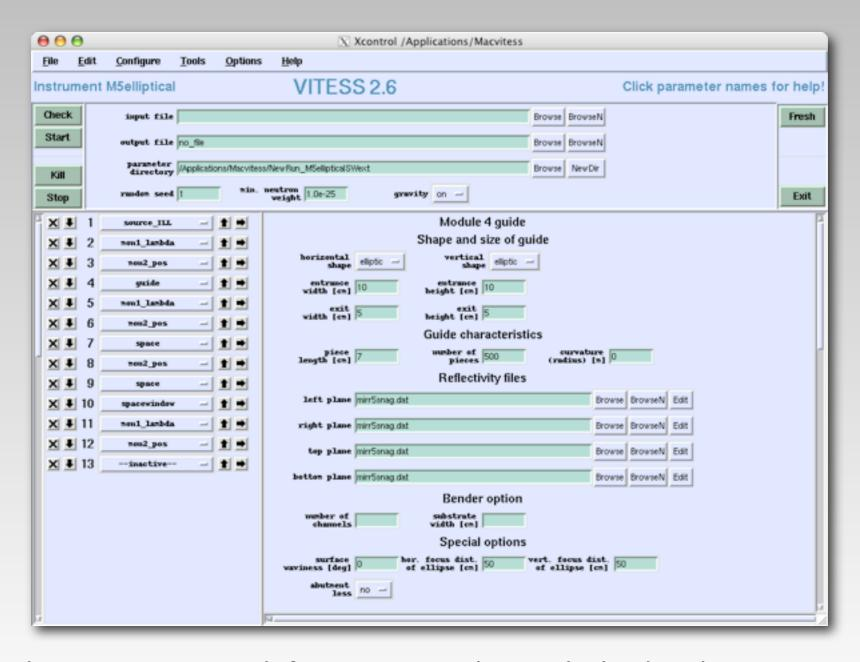
Monte Carlo neutron transport code for neutron scattering at pulsed and continuous neutron sources Extensively used to design and optimize neutron instruments worldwide
