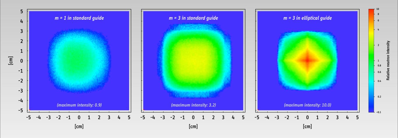
Shown are the planes of best focus behind the exit of a guide with a total length of 35 m Each simulation is based on 10 million neutron tracks
